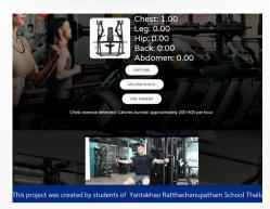
When the program is activated, the user clicks "Start" to use the camera to take a picture of the exercise machine or clicks "Upload" to upload an existing image. Afterward, the system analyzes the image to identify the type of exercise machine, displays a message showing the estimated calorie burn, and shows a sample video demonstrating how to use that exercise machine.
